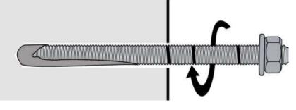
pushes the resin into any voids in the hole.
